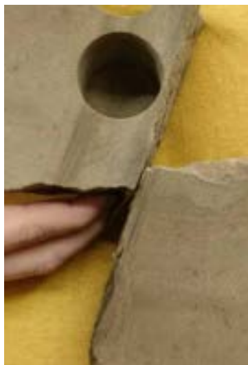
Figure 13: Open fractures associated with deformation bands in Ormskirk Sandstone core from the Douglas Field
